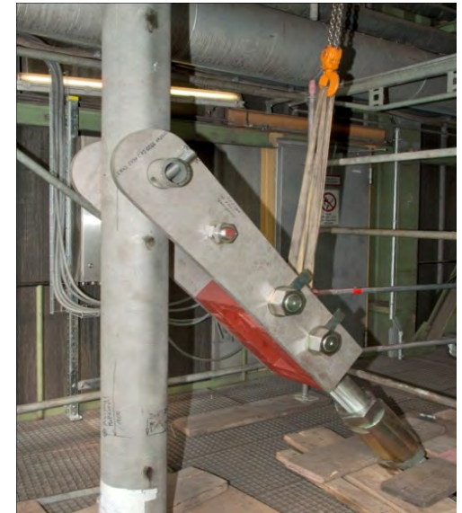
„Biegebremse“: Secondary stresses in pipe bend
